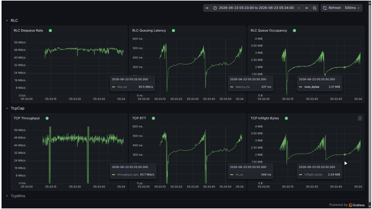
Figure 4.1: Grafana dashboard showing real-time RLC and TCP telemetry collected by RATO and TcpCap.
